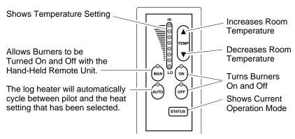
Figure 28 - Thermostat Hand-Held Remote Control Unit Selections
